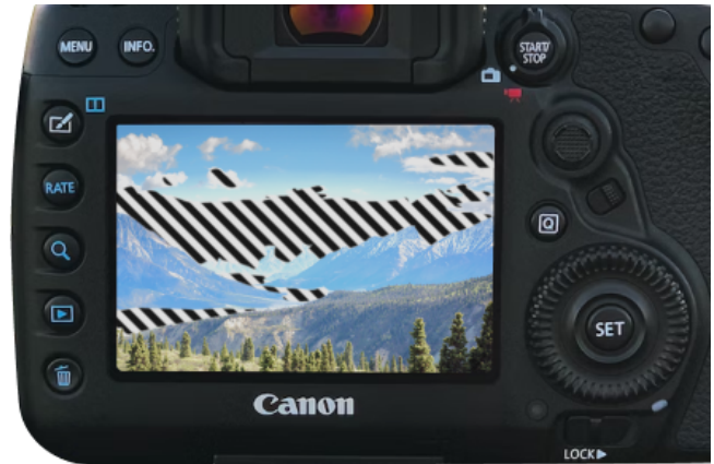
Figure 2: Examples of highlighting. The camera highlights over-exposed areas of the image with an animated zebra pattern. Furthermore, this caption draws the reader’s attention to the zebra pattern instead of the camera’s buttons. Image from Unsplash by Ben Griffiths.
